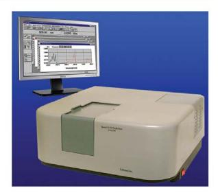
Spectro UV-VIS Double Beam UVD 3500 Research Spectrophotometer is a superior instrument for the research laboratory and is an advanced and affordable system that generates accurate and reproducible measurements. UVD-3500 spectrophotometer is accurate, reliable, and an exceptional value. With its narrow beam design, the system provides optimal and reproducible results for micro and macro samples with high resolution.
